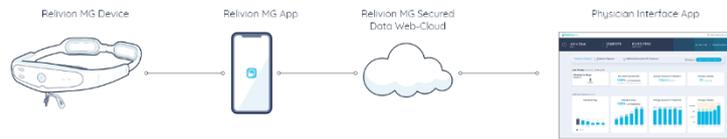
Figure 18: Relivion MG PMI Communication Flow
